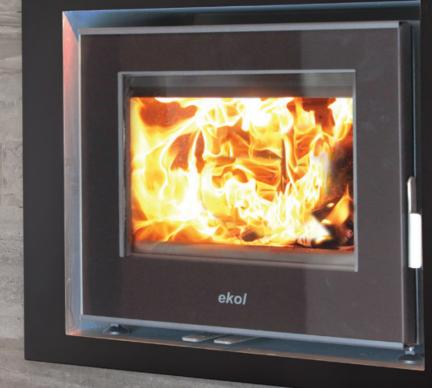
The Adept has a much shorter install time compared to most inset / 'cassette' type stoves -This is due to the integrated dual layers of thick steel which make up every Adept stove. Simply fire-board out the aperture in the wall, slide the Adept into the recess keeping 30mm gap all around, then connect the flue from inside the stove.
