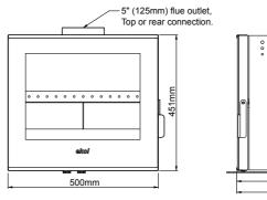
All air is introduced through rear air-intake which can if required be connected to outside air via 3" or 4" ducting. (Optional air intake from underneath is available if required)
