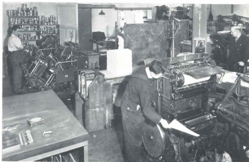
A section of the platen machine room which produces printed sheets up to a paper size of 19½" × 12½"
