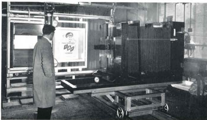
A double-crown camera (30" x 20") with copy being photographed through a prism attachment.
