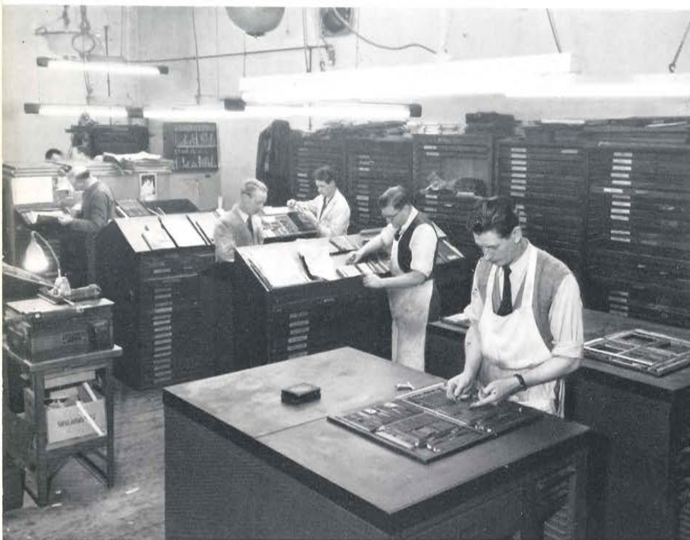
Typematter being imposed in a steel chase for the printing machine. It is then known as a forme.
