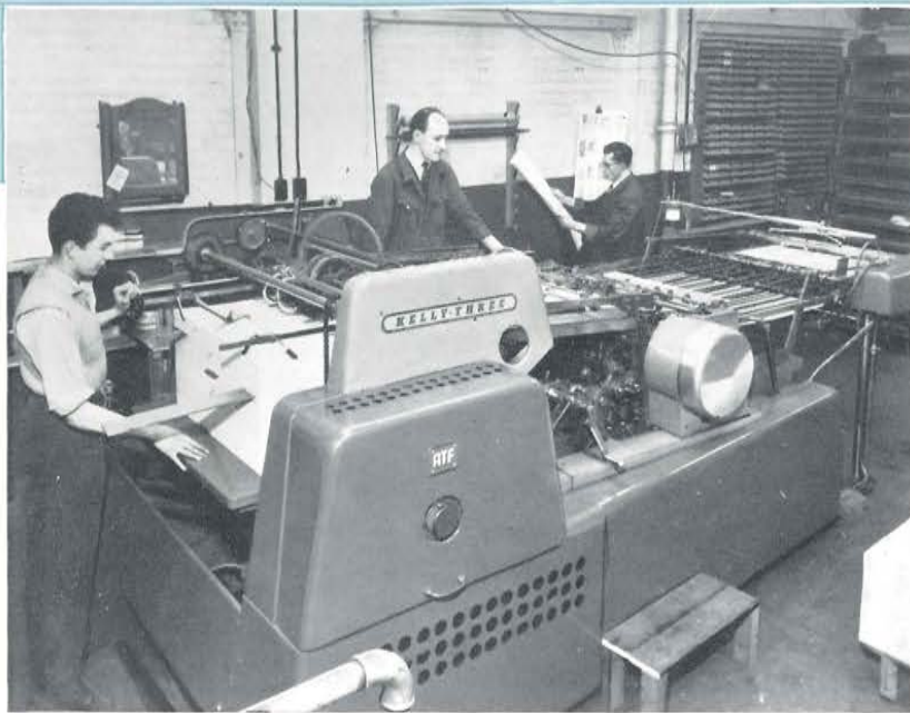
Before the machines start to run, many hours may have to be spent making ready to obtain perfect clarity of type and correct tonal values in the illustrations. Here, the Overseer examines a made-ready sheet.
