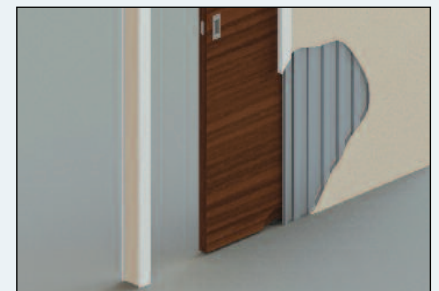
Timber door jamb c/w dovetail sheet corrugated cassette with plasterboard and concealed floor guide
