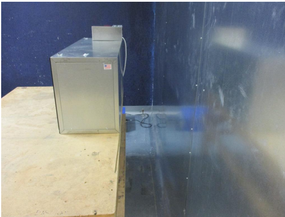
Figure 7-2 Conducted Emissions Test Setup Back
