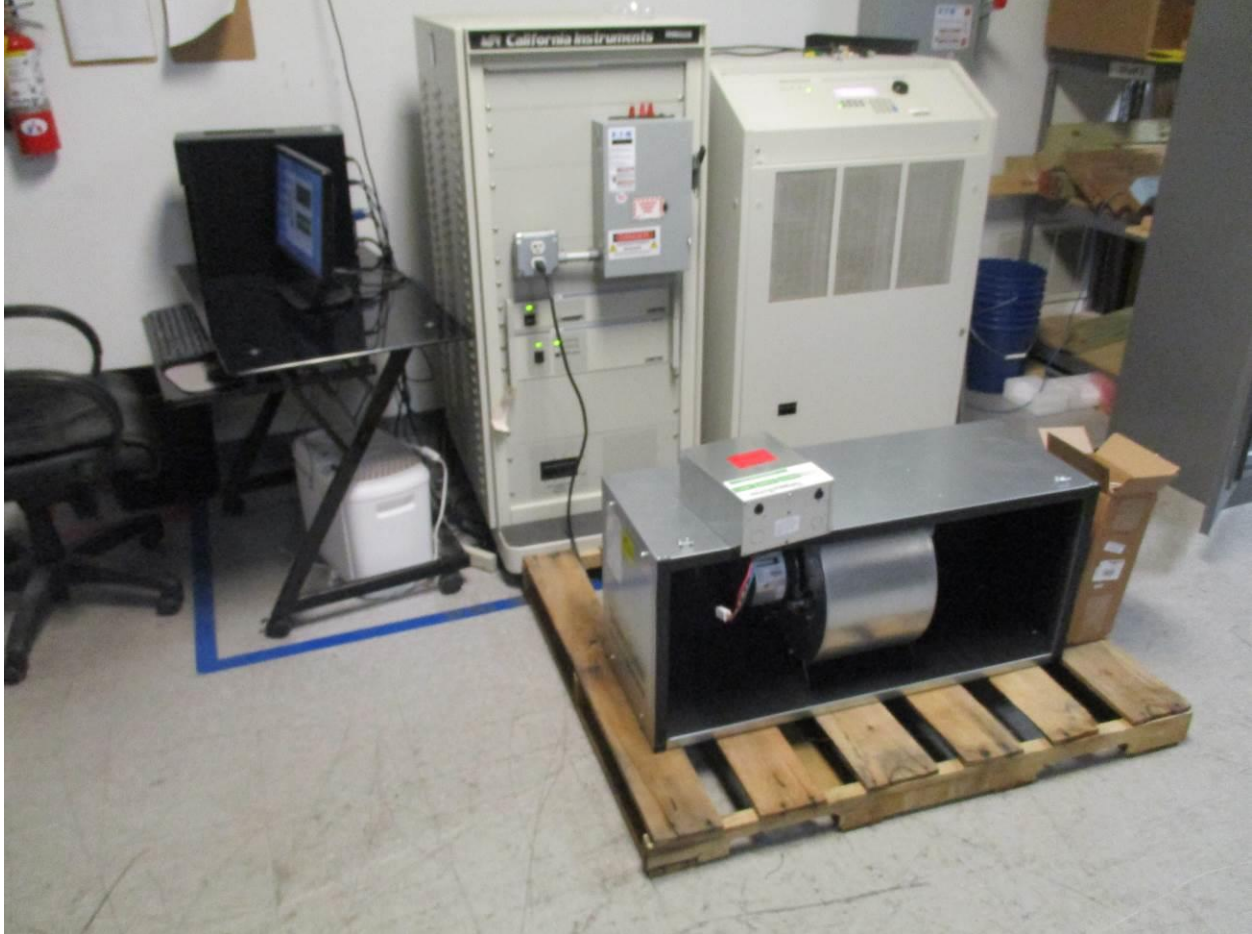
Figure 8-1 Harmonics Test Setup
