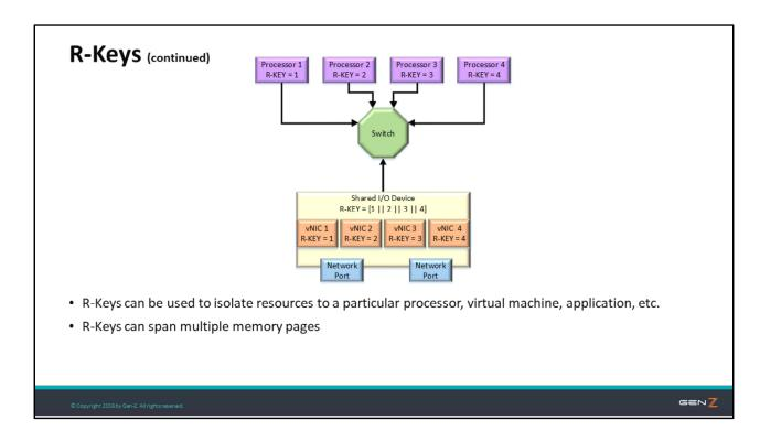
In this example, multiple processors are simultaneously sharing an I/O device (e.g., a Gen-Z Logical PCI Device (LPD)). Each Requester application uses a distinct R-Key to access the corresponding virtual NIC resources. Components that take advantage of Gen-Z's architecture, e.g., multipath, R-Keys, etc. can safely share a Responder without fear that their resources will be compromised by a peer component's access.
