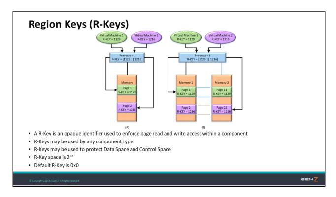
An R-Key is a 32-bit opaque identifier used to validate access permission to an addressable resource at page-level granularity. R-Keys are managed by application or middleware software.
