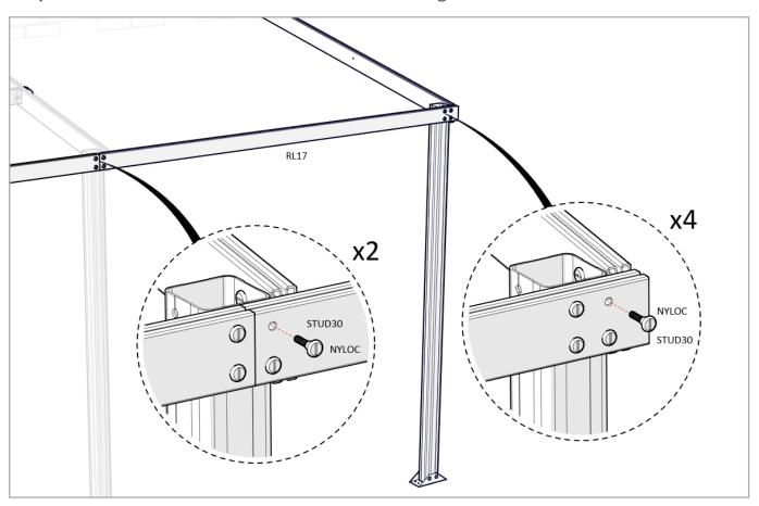
Step 6 - Fasten 2x HBD brackets to BM1 as shown
