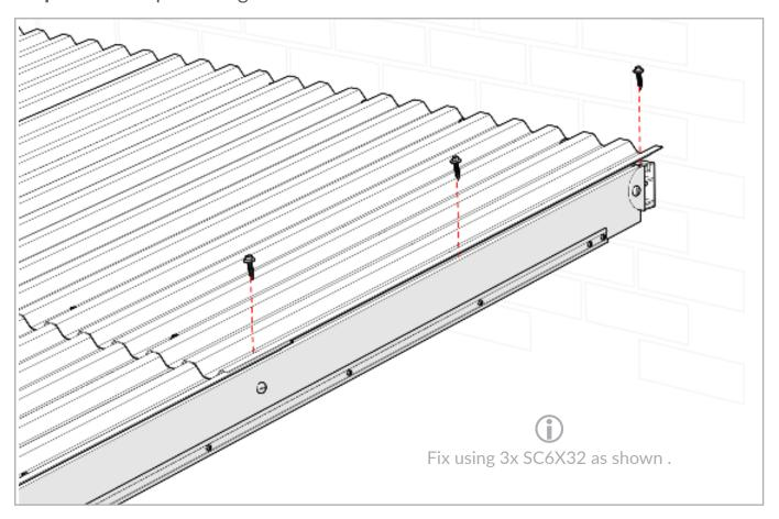
Step 18 - Assemble gutter and fix to front beam of carport
