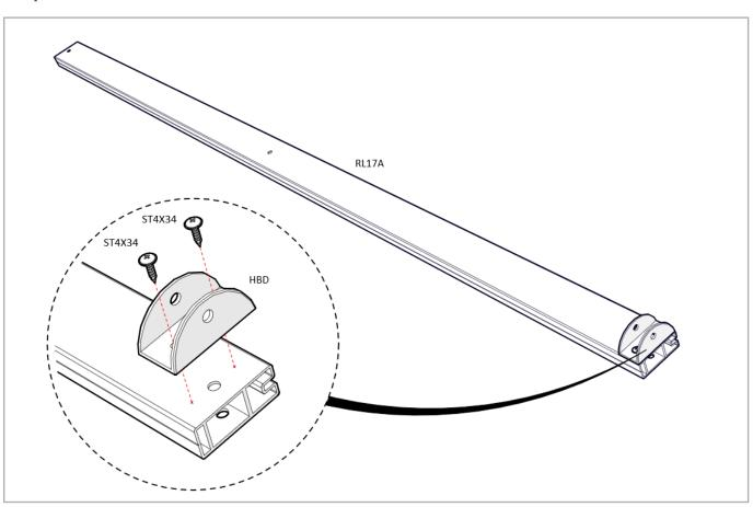
Step 3 - Fix RL17A to wall level with existing wall beams
