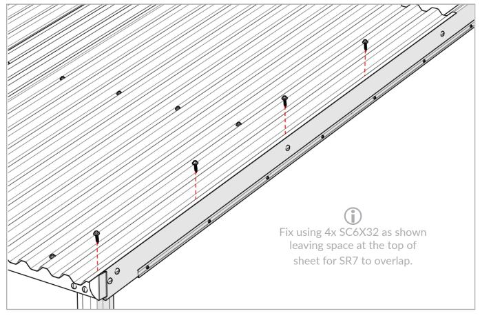
Step 12 - Position SR7 on top of first SR6, tight against the wall and fix.
