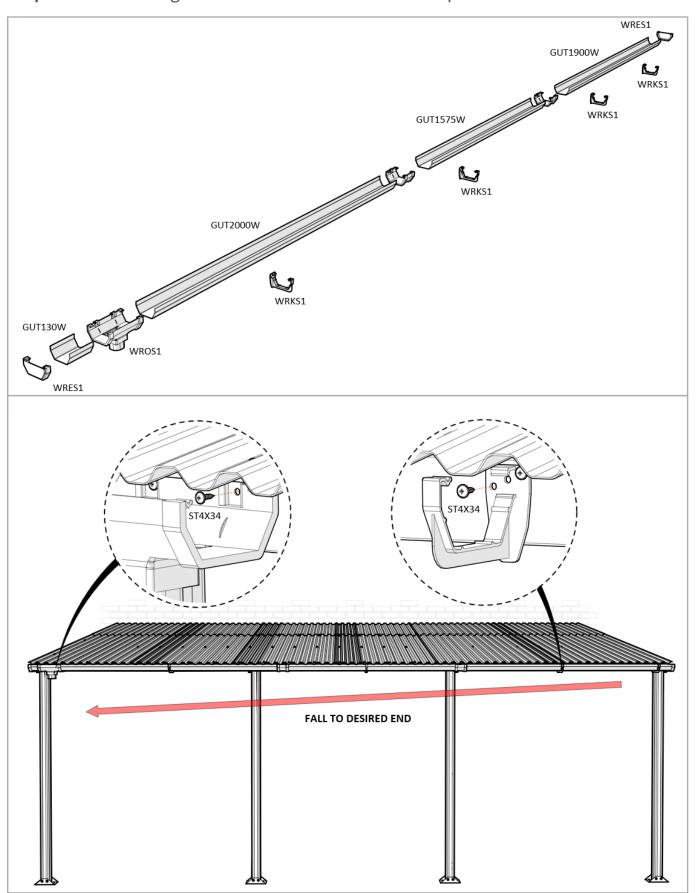
Step 19 - Assemble and fix downpipe to LEG
