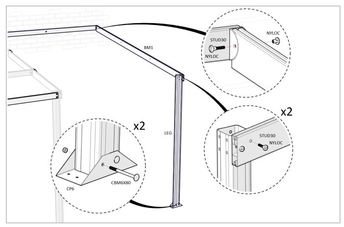
Step 5 - Fix RL17 as front beam between existing structure and LEG
