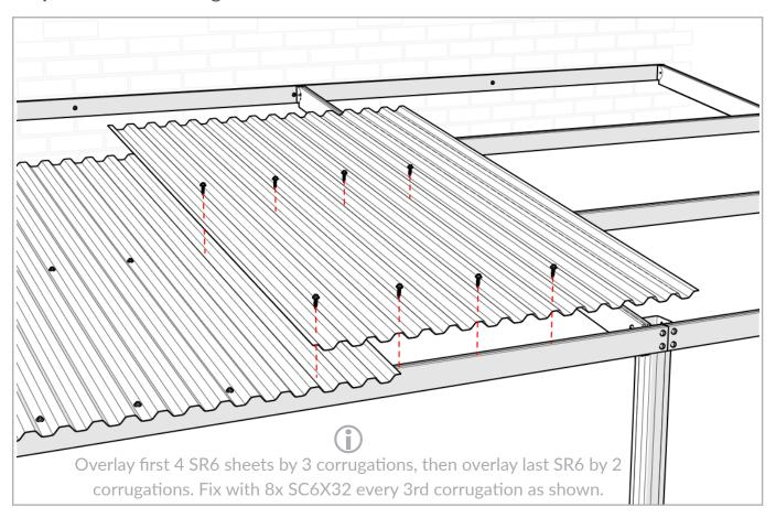
**Step 11** - Fix exposed edge of last SR6 sheet to BM1
