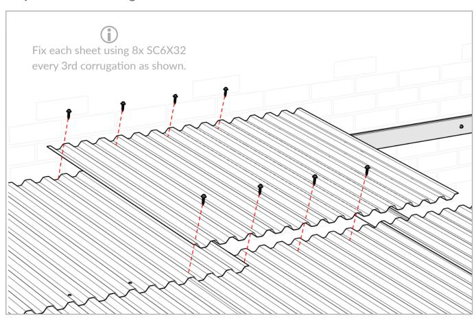
**Step 17** - Fix exposed edge of last SR7 sheet to BM1
