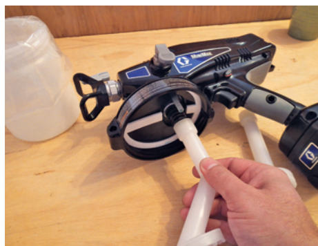
▲ Two different suction tubes are supplied – these simply push on
