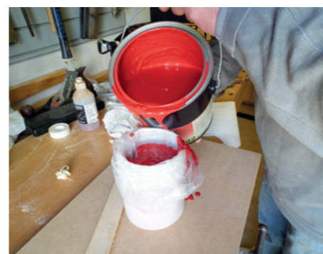
▲ A simple polythene bag serves as a liner to minimise clean-up after spraying
