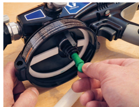
▲ Inserting the green plug restricts the flow of thinner fluids to avoid runs and sags
