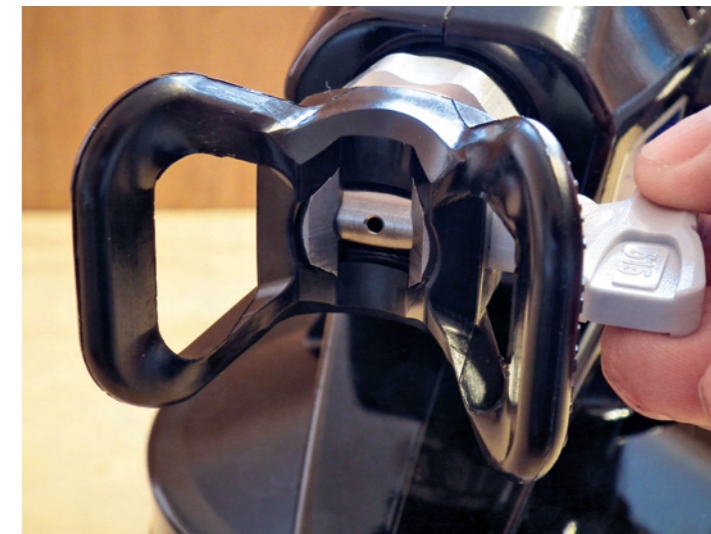
▲ The nozzle rotates through 180° to allow easy unblocking
