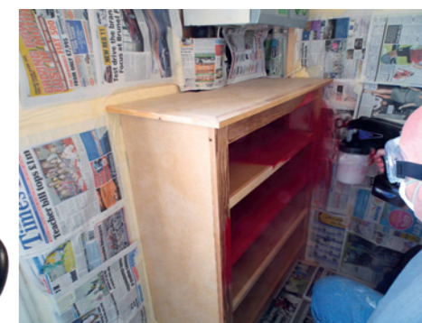
▲ Though an effective performer, this is an 'all or nothing' gun – you can't control the amount of output in the usual way
