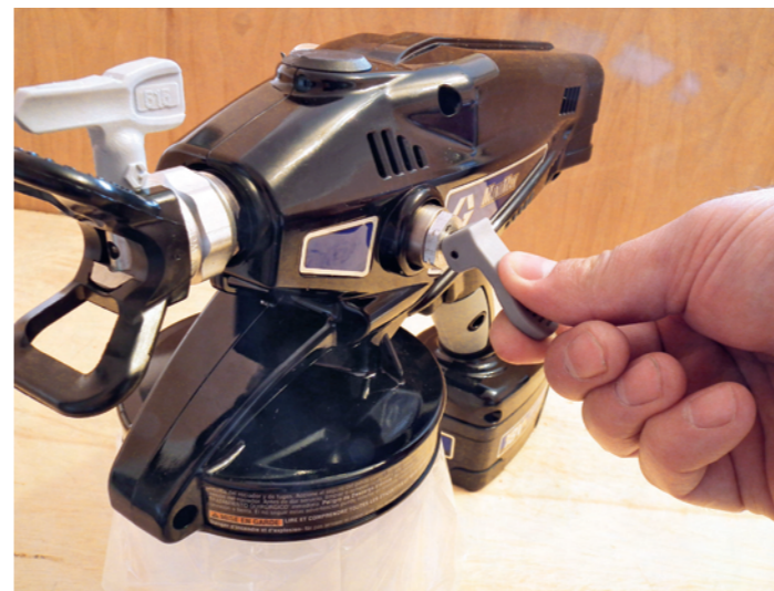
▲ The priming lever is used to get the paint into the gun or to release pressure
