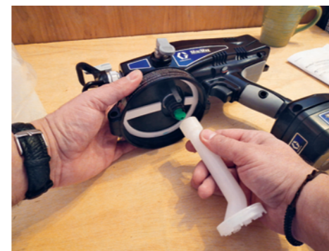
▲ The suction tube is then placed directly over the plug
