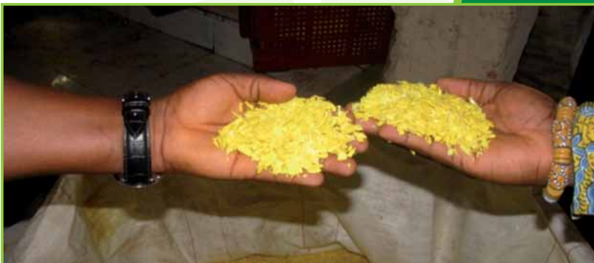
Shredding of cleaned empty containers in Ghana
