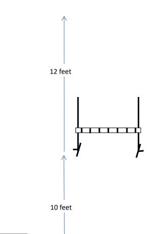
Sign is placed about 2 feet to the left of and at least 10 feet before the jump when used with sign 416.
