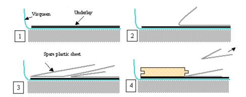
Whilst laying the floor, the floor fitting foam can be slightly stretched before sticking down the boards. So, if the boards shrink slightly they will tighten up to avoid gaps.
