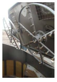
Washing rotor with rotating high-pressure water jets
