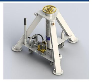
The Model 8955 Tripod Jack is a 10 ton capacity single stage hydraulic jack designed for use in aircraft maintenance. It consists of a tripod structure with integrated dual-leg reservoirs, hydraulic cylinder assembly, hand pump, swivel casters, locknut with handwheel and optional air pump with remote air inlet for remote air manifold operational control and a deadman air valve for individual jack operation.
