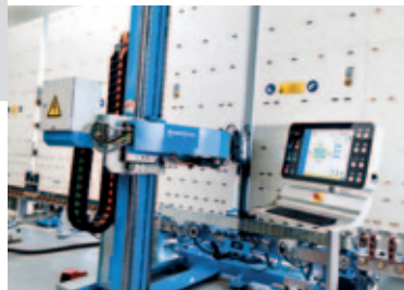
EDGEDELETER Coated glass plate edge deletion
