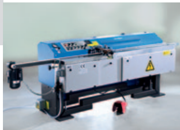
BUTYLEXTRUDER Double-sided coating of spacer frames with thermoplastic sealants
