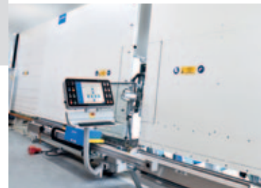
SEALER Entry solution for automated sealing of insulating glass units
