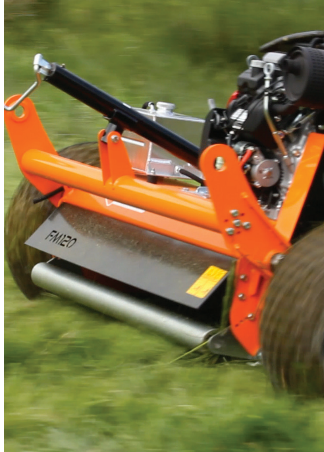
Wheels trailing the machine (to enable cutting close to hedges and fences).
