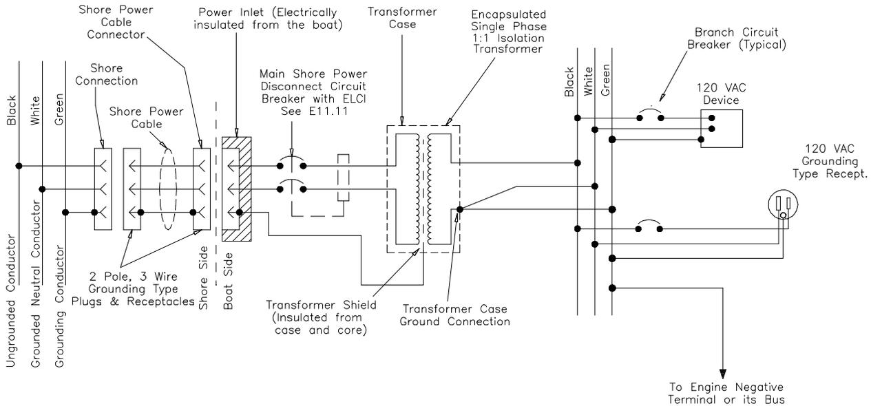
**11.17.5** Isolation Transformer System with Single Phase 240 Volt Input, 120/240-Volt Output with Boat Grounded Secondary. Transformer Shield Grounded on the Shore. Transformer Metal Case Grounded on the Boat. (See [DIAGRAM 7.](#))
