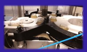
This solution allows the engineer to position the required guides onto the locating pillars, then lift and twist the handles to lock the guides in place.
