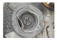
Wheel and tyre damage – no doubt the air loss was caused by rim damage. However it is necessary to examine the interior of the tyre to see if there is any evidence of pre existing punctures or run flat damage.
