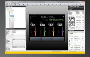
The Target View is the WYSIWYG screen design and layout area for a GUIX Studio embedded user interface. It is the "canvas" on which the GUI is designed. Objects can be selected, moved, resized and more via simple, intuitive mouse operations. In addition, alignment and Z-order button operations are available in the Target View.
