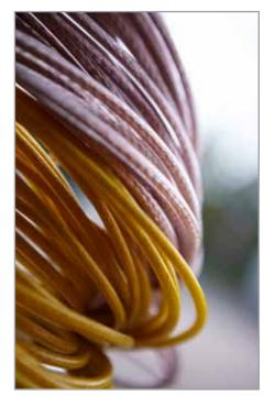
So how many wires make up a stranded wire? The answer depends upon the application. More strands means more flexibility and greater resistance to kinking or breaking, resulting in a stronger wire.
