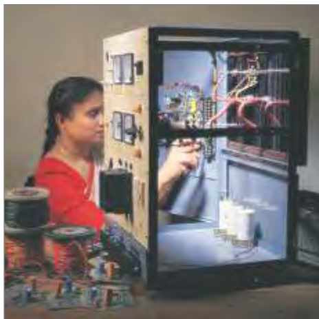
A constant current, constant voltage charger under manufacture.
