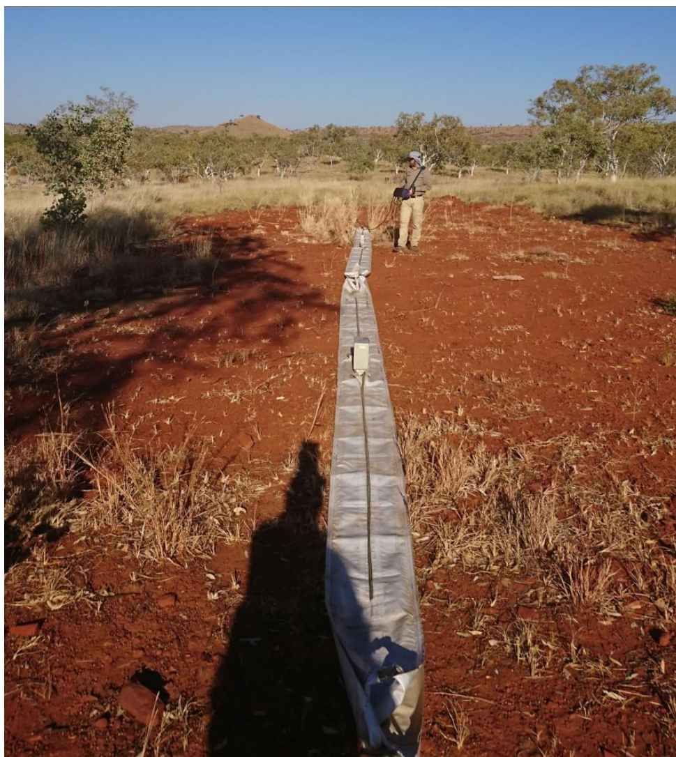
Figure 5 – Manually towed GPR sensor & transmitter array on location, southwest EL24451, July 2018.
