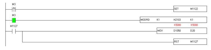
Using M1127 we can reset the flag when sending and receiving of the data is complete.
