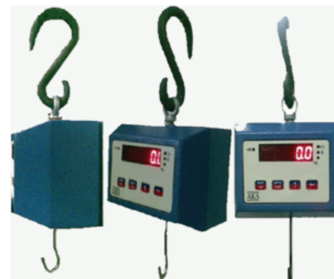
Figure 13: Example of an electronic weighing machine. Whilst its design and readout are simple, it has interlinked Bluetooth, which allows weights to be transmitted to mobile devices
