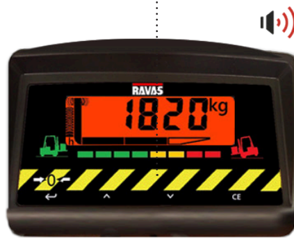
Overload situation: tip loading
