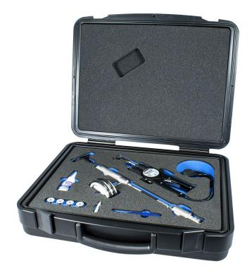
Supplied in an industrial foam-filled Carrying Case with 5 Flat Dollies, Adhesive, Heated Dolly Remover, Dolly Cleaning Tool and Dolly Plug.
