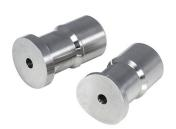
The Adhesion Tester can test both external and internal surfaces of pipes. Because the load reacts internally within the dolly, curved surfaces of pipes can be easily tested.
