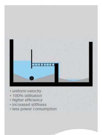
In a vertical configuration, only the bottom section of the screen is used during periods of low flow, and flow velocity is significantly higher. With a horizontal configuration the entire screen is used, no matter how high or low the flow. Flow velocity is kept to a minimum and the need for secondary weirs is eliminated, preventing grit and heavy solids from becoming trapped and so reducing the screen's efficiency.
