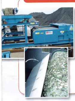
Eddy Current Separators are increasingly used wherever separation of non-ferrous metals from a product stream can give a more valuable end product. Whether the end use is in recycling, waste reduction, raw material production or any other process where separation would prove beneficial. Typical examples of applications are:
