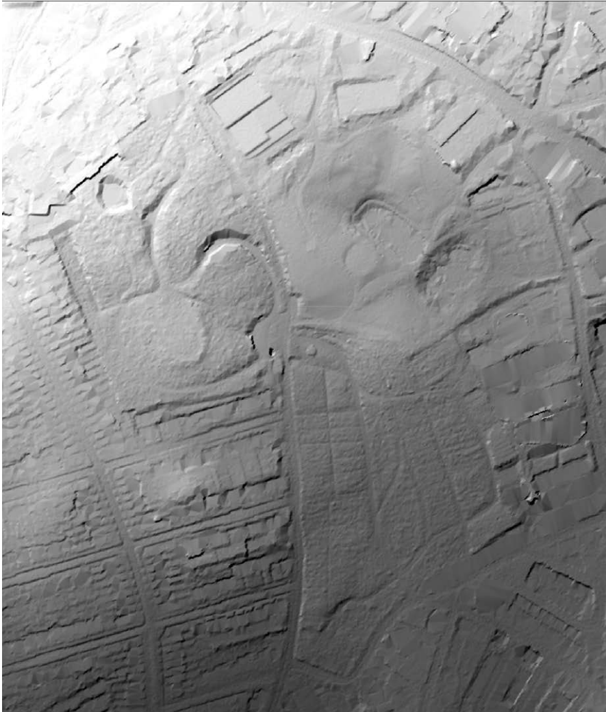
Fig 11. Environment Agency LiDAR survey, showing terrain at 1m resolution (Environment Agency, 2017)
