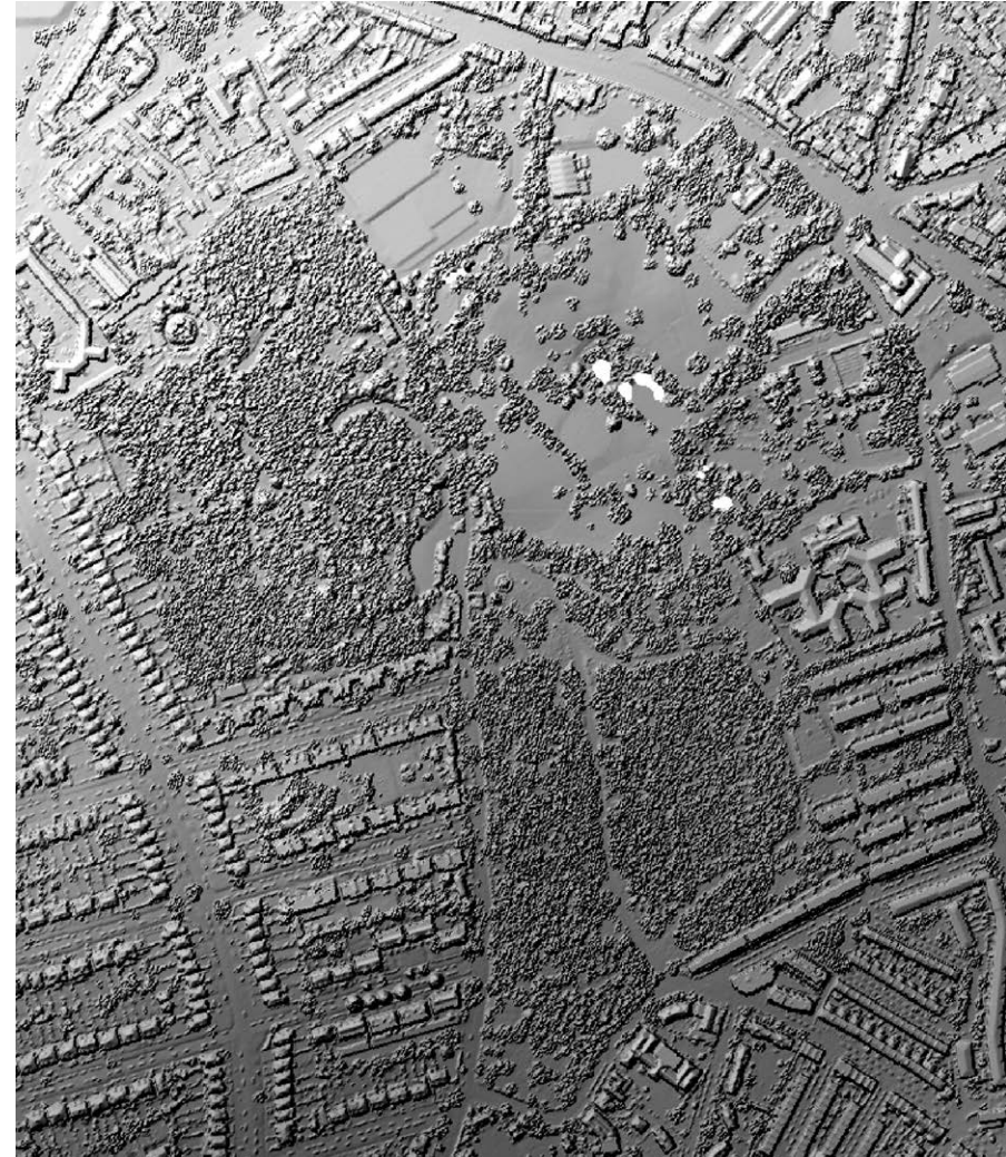
Fig 12. Environment Agency LiDAR survey, showing surface features at 1m resolution (Environment Agency, 2017)
