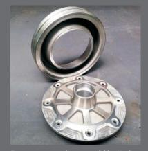
Precision machining of the hub incorporates off the shelf automotive bearings for quick and inexpensive replacement when needed.
