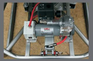
The Helispread system uses high quality and readily available commercial air cooled compressors fitted complete with a control box available in 12 or 24v drawing on average 12–13 amps from the aircraft when in use.
