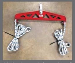
A hook and go spreader bar complete with certified nylon flexi-rope significantly reduces lifting shock on take off when the bucket is full.
