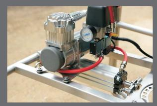
Helispread only uses high quality Pneumatic air rams that will provide years of trouble free service for the operator. Interchangeable orifice plates allow the operator to determine product application rates per hectare/acre.
