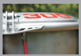
Only the Helispread system has an inbuilt precharged air reservoir delivering 100% performance to the Pneumatic actuator for rapid and instant opening and closing of the hopper gate.
