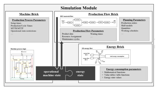
Figure 5: Conceptual structure of the simulation module.
