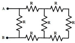
*The November Bonus:* if the resistances R in the circuit above all equal 15 ohms, what is the resistance between contacts A and B?
