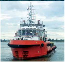
In FY2011, we have grown our fleet of young vessels. In all, we have in our fleet Vallianz Hope, a 4,200 BHP anchor handling tug supply vessel, 40 metres in length; Swiber Bhanwar, a 4,750 BHP anchor handling tug that is 48 metres in length; Swiber Carina, a 2,400 BHP Utility Vessel that is 40 metres in length; Swiber Charlton, a 3,200 BHP towing tug that is 33.2 metres in length and Swiber Raven, a 3,200 BHP towing tug that is 31.1 metres long.
