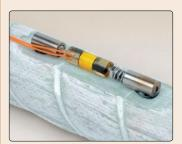
Model 4151 Strain Gage mounted to a fiberglass rebar.
