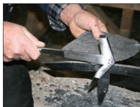
Picture illustrates slate hammer mid-section being used to trim slate utilizing a stake as base.
