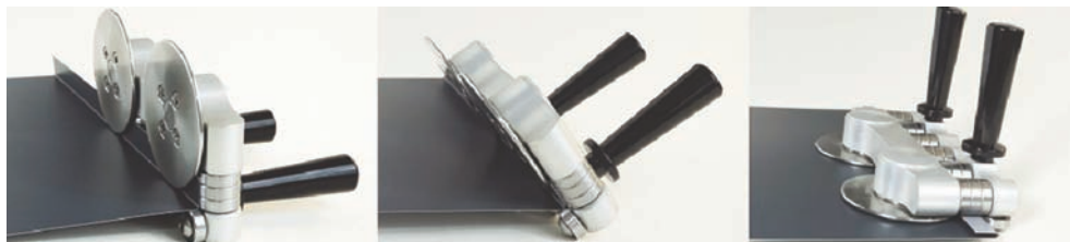
Bending example #2: The model XL hemmer takes the 90° bend down to 180° in a few passes
