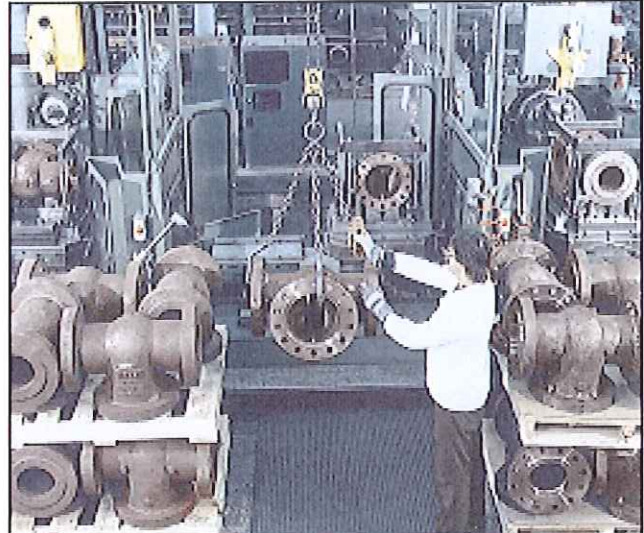
For smaller runs, complete automatic machining and drilling in one set-up.
