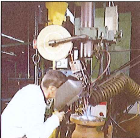
1 Automatic seal welding of Stellite 6 hardfaced seats.
