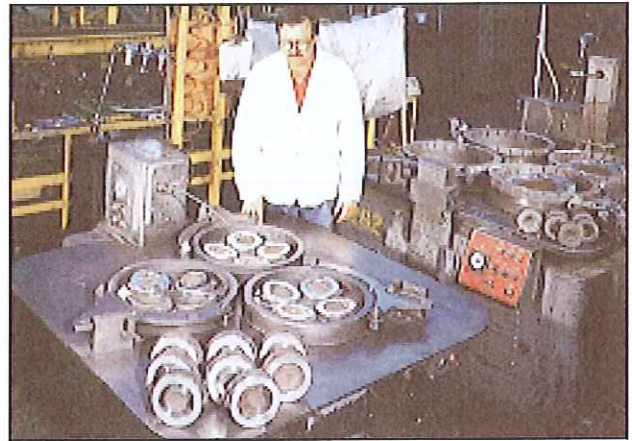
6 Lapping of wedge seating surfaces.
