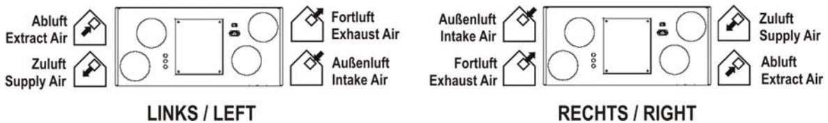
Figure 24: Tag of the connection of the air ducts
