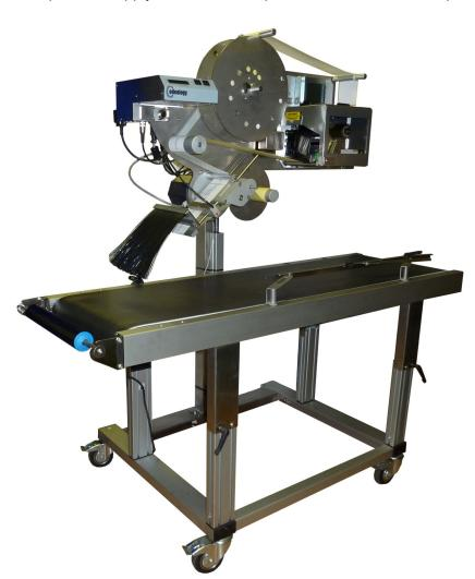
The P150 is simple, robust and low-cost. We keep the cost down by using a proven dc motor drive system that has already been shown to be long-lasting through years of use in our P100 side print-and-apply systems..
