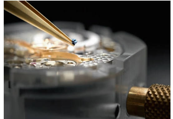
CLOCKWISE FROM LEFT: a craftsman adding a whiplash spring; the man who brought A. Lange & Söhne back from the dead, Walter Lange; 'blued' screws, which have been hardened and given colour by heating, add a decorative touch to high-end clockwork
