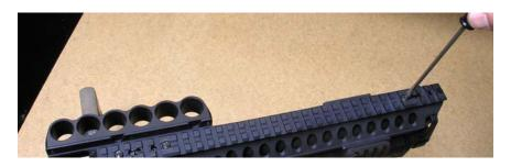
Now use the gold hex keys (blue in these photos) to fully tighten the M4 button head screws and the angled set screws.
