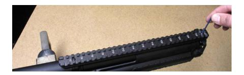
Once the screws are out, remove the rail:
