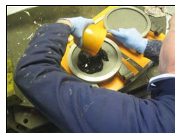
After application of Belzona 2221
