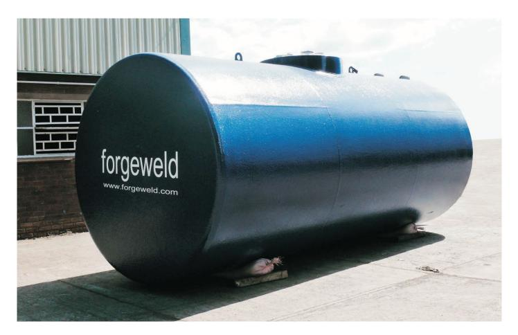
The tanks consist of a steel primary tank enclosed within a steel secondary tank. A 25-mm interstice is formed between the inner and outer tank. After tank installation, the interstice is filled with a mixture of water and glycol. Any loss of liquid level or pressure activates an alarm. The glycol mixture also provides insolation and temperature control.
