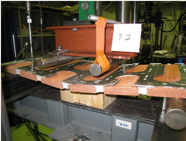
Photo 20. Failure at mortar joint.
