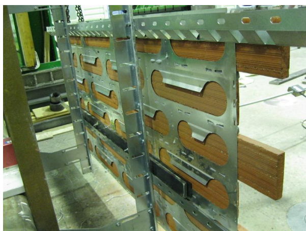
Photos 6 and 7. Load was concentrated on backside with the help of rubber strips (300 mm long) to fixing areas of horizontal rails.
