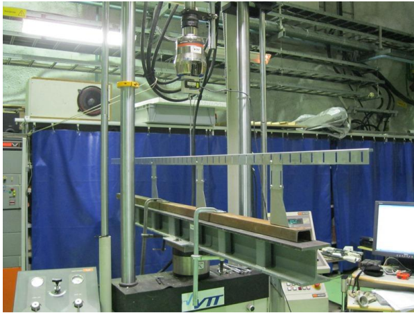
Photos 1 and 2. Test arrangements, loading point 70...130 mm from the fixing screw.
