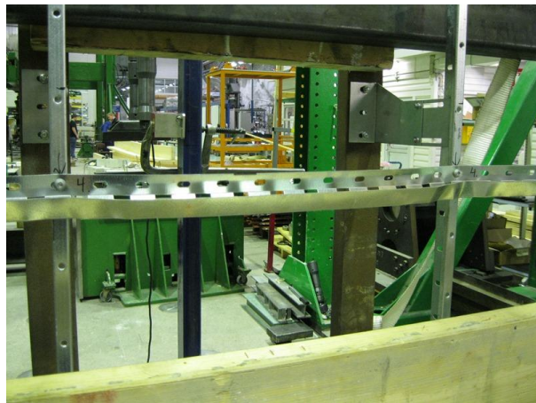
Photo 13. Horizontal rail after failure.
