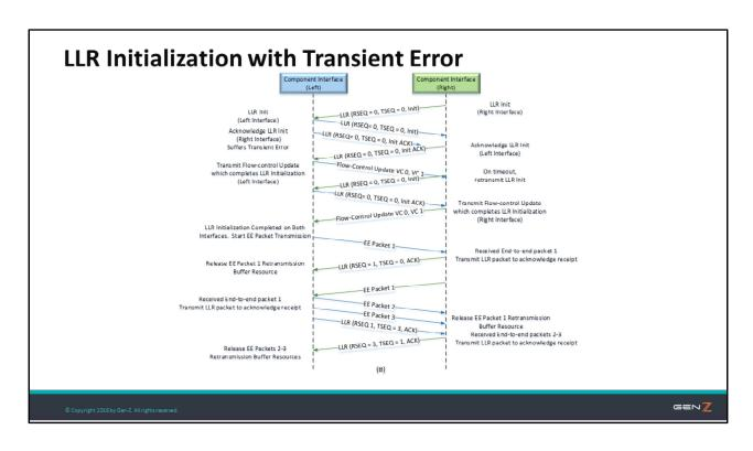
This slide illustrates LLR initialization where the LLR Init ACK transmitted by the left interface is lost due to a transient error.
