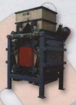
High capacity separators for the concentration of finely sized paramagnetic ores and for the purification of non metallic minerals.
