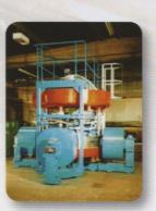
Wet High Intensity Mineral Separators are used for the continuous extraction and concentration of fine paramagnetic materials presented in a wet state.
