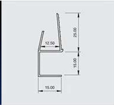
Locally manufactured from recycled plastic, Renderplas PVCu architrave shadow gap beads are designed for plasterboard to quickly and accurately form a shadow gap and provide a superior clean finish. Used at the edges of the plasterboard next to door frames, ceilings and skirting boards where the adjacent finish is hidden
