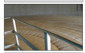
Stage 3 From the steeping vessels, the chitted barley is transferred to a Germinating and Kilning Vessel (GKV). Inside the GKV the barley is allowed to germinate in conditions of controlled humidity (shown above) with regular gentle "turning" of the metre-deep grain bed to prevent matting. The GKVs at Simpsons utilise a rotating floor and fixed turner beam to assist with the loading, turning and unloading of the product.
