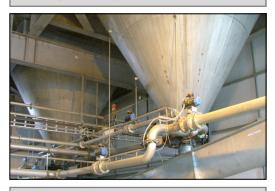
Stage 2 The barley is transferred into stainless-steel cylindrical steeping vessels (above) where it is steeped in natural water from boreholes. Low-pressure air is pumped through the vessel at regular intervals to keep the individual grains separate, until the root tip (or "chit") appears at the end of the grain.
