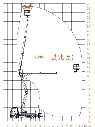
The Z26 takes the highly versatile sigma/telescopic boom geometry onto a 7.5tonne chassis. Almost 26m working height with up to 12.5m of up and over outreach with zero tailswing from a narrow 2.8m outrigger width. The Z26 offers the proven 'Z' control system of its smaller relations: simple proportional controls, basket load sensing, load sensing outrigger interlocks and zero tailswing. The Z26 is also fitted with automatic self-levelling outrigger option for the UK.
