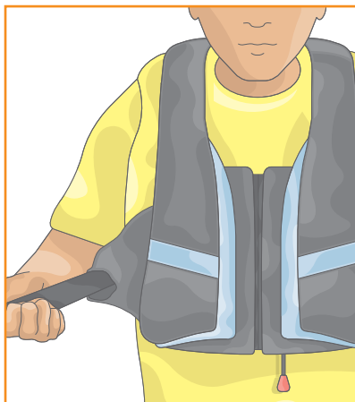
The straps are 'rocked' forwards and backwards to obtain a tighter fit
