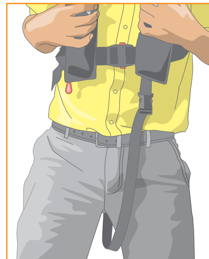
Crotch strap too loose
