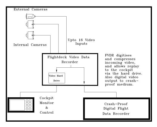
Figure 2 - Crash Proof Flightdeck Video Data Recorder
