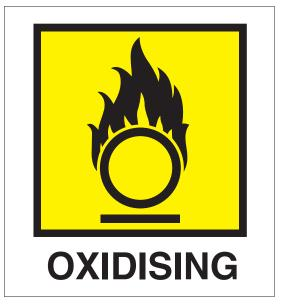
Figure 4: Label on oxidising materials
